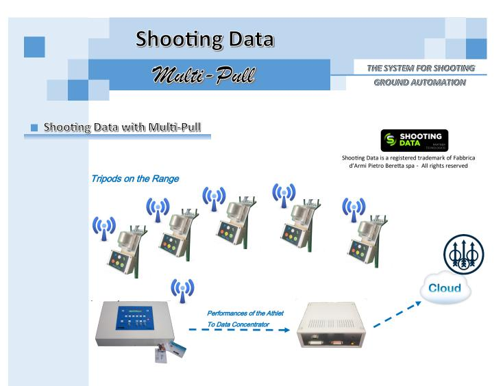
To use the Shooting Data system with the *Multi - Pull* it is necessary to install on each tripod of the **EP096AT** series some wifi modules model **EP096RFID**. These modules are able to communicate with the **EP095M** control unit via wifi.
